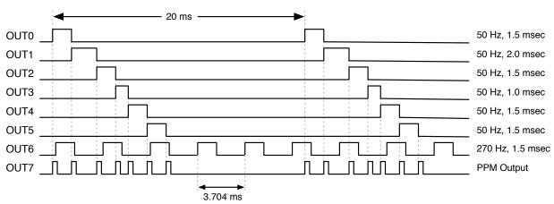
Note: Outputs that use the alternate frequency are not included in the PPM output (only 50 Hz outputs).
